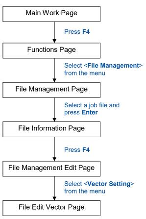
The File Edit Vector Page allows you to edit the vector pen, vector power, vector speed, and vector PPI, and power ramp settings for the selected job. These settings correspond to the same settings found on the LaserPro T500 print driver. This page allows you to easily adjust these values to make immediate adjustments while processing your loaded jobs, even when you have disconnected your computer from the LaserPro T500.
