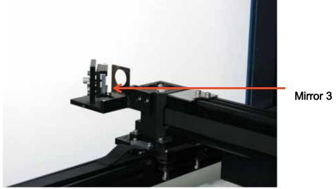
(Figure 8- 3 Cleaning the Mirrors)
