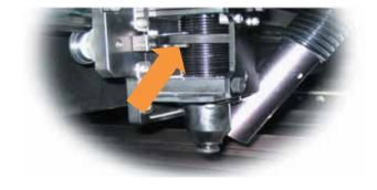
**4.1.9 Knife-shaped Cutting Table**Unique cutting table with tipped bars that can be easily adjusted without tools to create different levels of working depths. The cutting table of T500 reduces laser reflections and delivers clear cutting edge.
