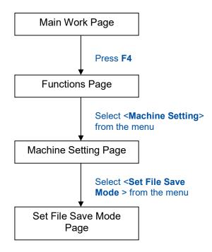
The Set File Save Mode Page allows you to set whether or not the LaserPro T500 automatically deletes each job file after processing. Setting File Save to <NO> will automatically and immediately delete each job file from the LaserPro T500 after the engraving or cutting process. Setting File Save to <YES> will retain all job files on the LaserPro T500, even after each job has been processed.
