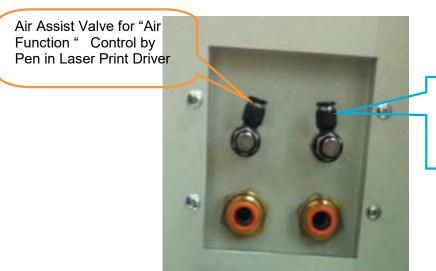
Air Assist Valve for preventing 150/ 200W laser tube from frosting
