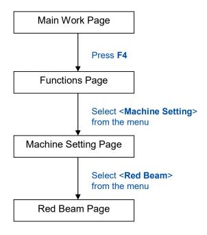
The Set Red Beam Page allows you to turn on or off the red dot laser pointer on the lens carriage. Enabling this function will indicate the exact area the engraving laser will fire upon.
