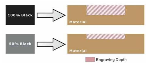
By specifying different levels of black in design software, the corresponding laser power energy will generate different depths of engraving result.
