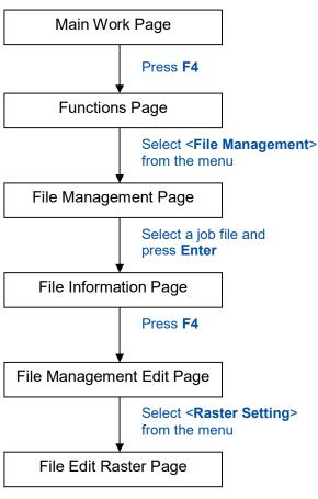
The File Edit Raster Page allows you to edit the raster power and speed settings, as well as enable or disable SmartACT for the selected job. These settings correspond to the same settings found on the LaserPro T500 print driver. This page allows you to easily adjust these values to make immediate adjustments while processing your loaded jobs, even when you have disconnected your computer from the LaserPro T500.
