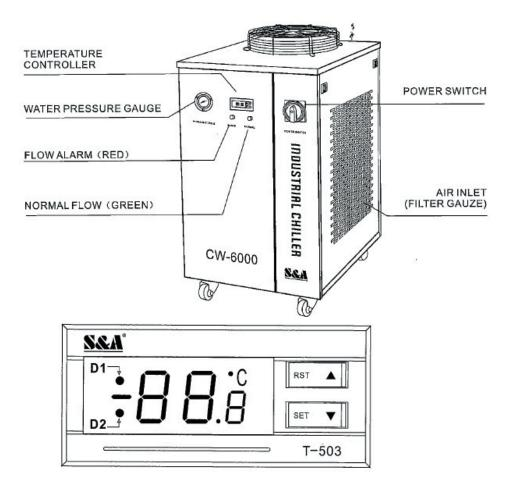
Turn on the chiller power switch, wait until the chiller compressor finished operation, and go for following setting and operation.
