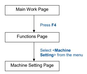
The Machine Setting Page allows you to access and modify a variety of your machine settings, including: Set Lens, Tune Auto Focus, Set Table Down, Set Red Beam, Carriage Lock, Set Command Mode, Save Position, Set File Save Mode, Set Vector Mode, Tune Image Power, Set Laser Wattage, Set Fine Mode, Other, and Reset.
