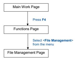
The File Management Page allows you to manage the files that you have loaded onto the LaserPro T500. You can scroll through your jobs, delete a selected job, delete all jobs, and go to the Link/DLink Page to set and arrange multiple loaded jobs into a single job queue for processing.
