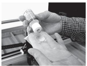
(Figure 8- 5 Cleaning the Mirrors)
