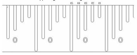
Place the Supporting Bars on different slot along with different focal lens, the acceptable maximum working piece will be varied. Please refer to below list.
