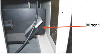
(Figure 8- 1 Cleaning the Mirrors)
