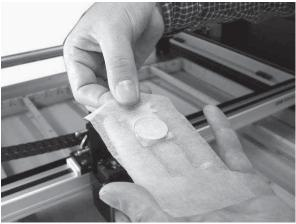
(Figure 8- 6 Cleaning the Mirrors)
