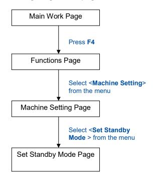
The Set Standby Mode page allows you to configure the laser machine automatically enter into power saving if machine is idle for a specified time.
