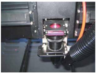
(Figure 8- 8 Cleaning the Focus Lens)
