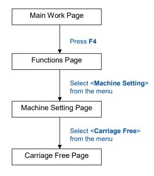
The Carriage Lock Page allows you to set whether the laser carriage is locked or free. If the Carriage Free setting is set to <YES>, then you will be able to manually move the laser carriage along the X and Y axis by hand with the top door open. Whereas setting the Carriage Free to <NO> will lock the laser carriage, and movement or positioning can only be done by the control panel.
