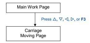
The Carriage moving page allows you to manually increase and decrease the height of the work table (Z-axis). In addition, you can manually adjust the Y-axis and X-axis of the laser carriage.
