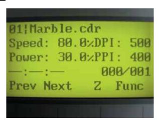
The main work page is the page that the LaserPro T500 will default to upon startup and will be the "home base" for when navigating through the various functions of the control panel. This will be the page that is displayed when you are processing your jobs. This page contains specific job information such as the current job's name, Speed, Power, PPI, DPI, processing / remaining times, and jobs loaded.
