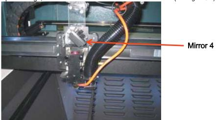
(Figure 8- 4 Cleaning the Mirrors)
