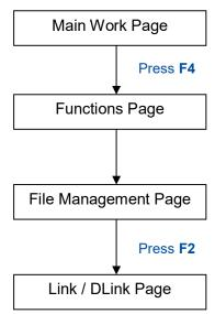
The Link/DLink Page allows you to set, arrange, and remove loaded jobs to and from a job queue for processing. Use the directional keys to cycle through your loaded jobs, then simply press the <F2 (Link)> key to add a file to the job queue. The job queue will be set in a sequential order based on the order you link the files. To remove a job from your job queue, press the <F4 (DLink)> key.
