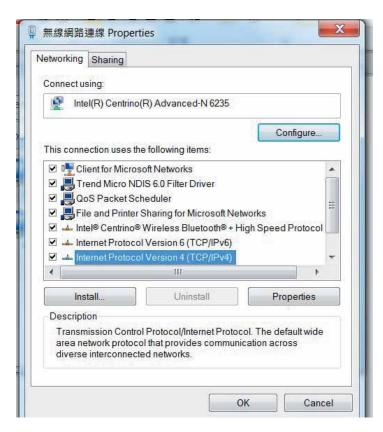
Step 7. Enter the IP address and Subnet mask setting values, and choose <OK> Note the IP address 192.168.3.X (X value can be 1~255, while can't be the same number as machine control panel setting in step 4)
