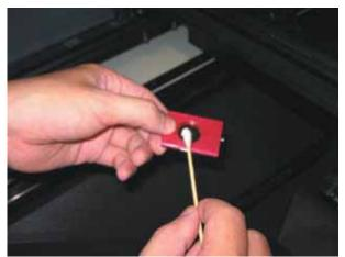
(Figure 8- 10 Cleaning the Focus Lens)
