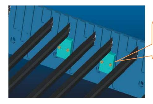
Supporting Bar Spacers reduce the cutting slot depth and create more slots in same level for supporting bars loading.
