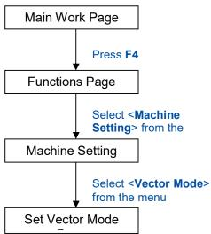
The Vector Mode Page allows you to adjust and balance vector mode's quality and speed settings based on your specific job. Speedy Vector Mode offers the highest output speed, sacrificing quality. Whereas Quality Vector Mode offers the highest quality, sacrificing output speed. Keep in mind that speed and quality are usually at a tradeoff. The system's default is Production mode, sacrificing some speed for higher quality. The LaserPro T500's default setting is <Production Vector>.
