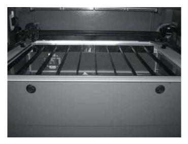
• Place the aluminum grid cutting table on the arranged supporting bars
