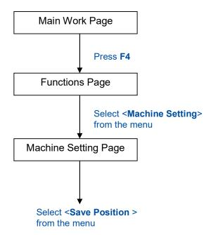
The Save Position Function allows you to save the current X-axis and Y-axis positions of the laser carriage and sets this position to be the origin for subsequent jobs.
