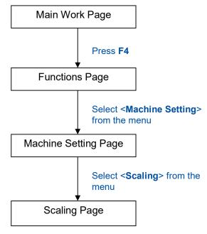
The Scaling Page allows you to fine tune the laser machine output scale to precisely fit the original graphic file design scale when precision output is required to your application.
