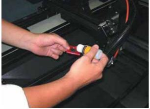
(Figure 8- 9 Cleaning the Focus Lens)
