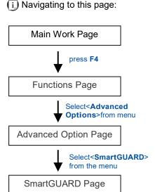
After optional SmartGUARD hardware installation, please enter the function menu on the control panel to enable the SmartGUARD fire alarm.
