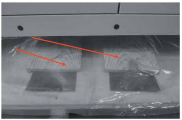
Step 7 Put the settled boards at each end of the crate base to form a slope.
