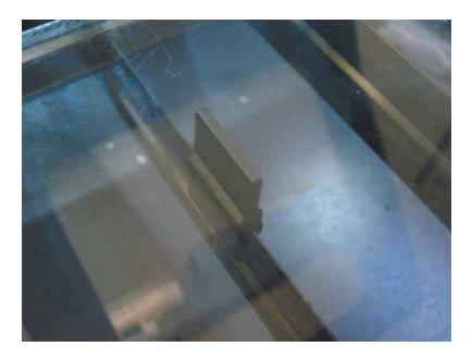
Apply the Position Mode in the LaserPro driver to process your cutting job at where you expect to be
