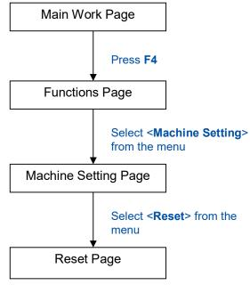
The Reset Page will restore machine settings back to factory default. Press ENTER to confirm the change, and restart the machine.
