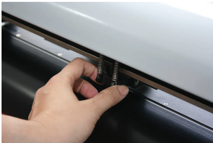
Figure 4-3 correct way to move pinch rollers
