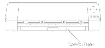
With the tray all the way out, flip open the inserted piece to reveal where you can place the roll feeder. There are two end pieces you'll also flip up, and this is where your rolled material will rest. Slide the right end piece to match the width of your material—either 9 inches or 12 inches.
