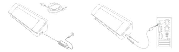
Next, connect your machine to your computer using the USB cable. Then press the circular power button to power on your machine.
