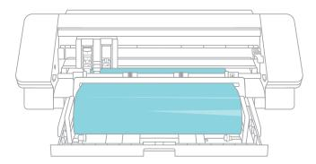
When you're finished using the roll feeder, remove the roll of material, fold the pieces back down, and slide the tray back into place.
