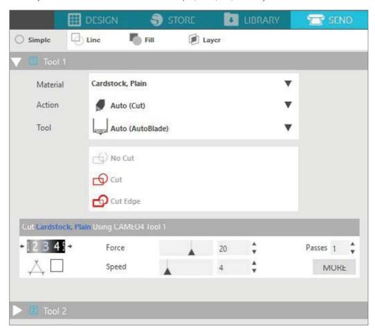
Each action allows you to adjust specific cut settings. Cutting is as easy as choosing your material, your action, and your tool in the Simple panel and clicking "Send."
