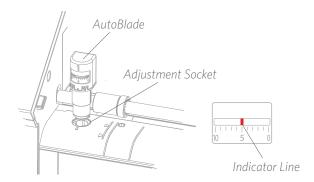
If you're using the AutoBlade, the blade will automatically adjust when you send your design to cut. To adjust the AutoBlade or any other blade manually, use the adjustment socket in the machine or the handheld tool that your machine comes with. Gently press the blade up and down into the adjustment socket until the red indicator line points to the desired setting.
