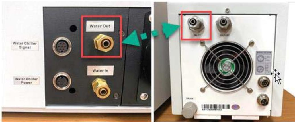
b. E200 machine "Water in" to water chiller "Outlet"
