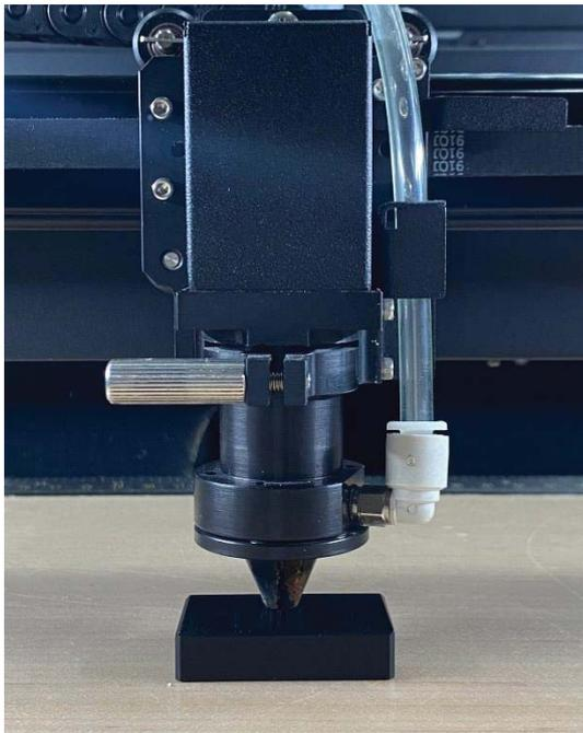
3. Place the focus tool between the material and the carriage, the following picture shows the focus distance with the nozzle installed.
