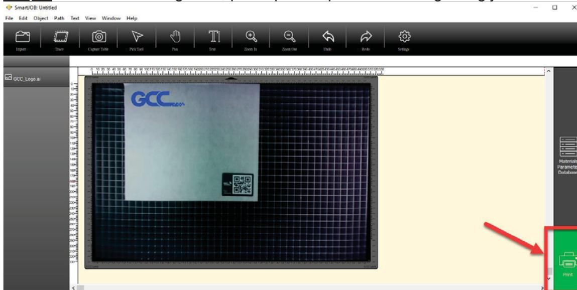
**Step 7** If you have adjusted the parameter, you can save the parameter into the material database and name it yourself.
