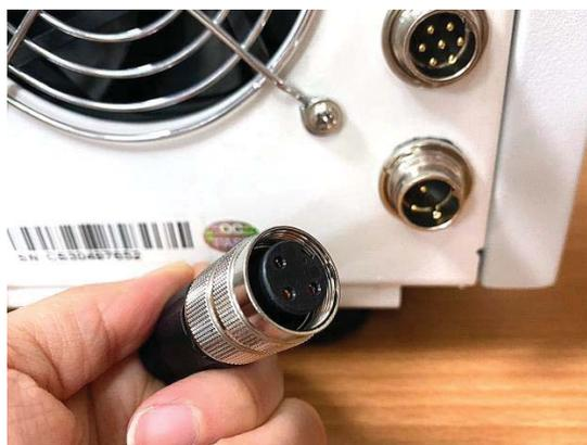
1) Connect the signal cable from the machine to the water chiller.
