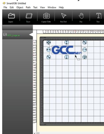
**Step 3** After loading the file, please click “Capture Table” to take a photo of working table and E200 camera will scan the barcode which stick on the GCC materials.
