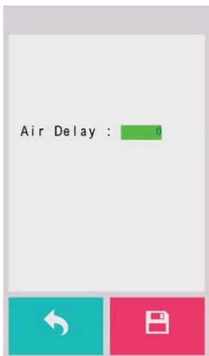
The Air Delay setting allows you to specify the delay in seconds of the SmartAIR air-assist after the point of laser firing.
