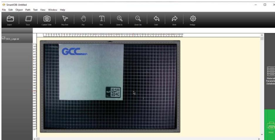
**Step 5** Go to file list, and click the right mouse button, SmartJOB will set up the parameter according to different materials automatically.
