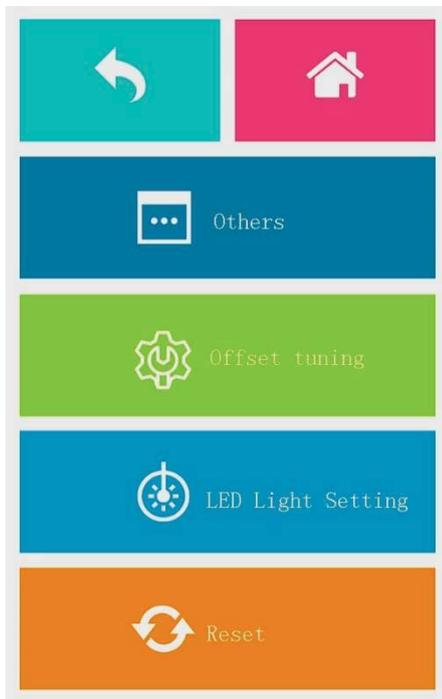
The Machine Setting Page allows you to access and modify various machine settings, including: Others (Air Delay), Offset tuning, LED light setting, Reset.
