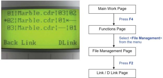
The Link/DLink Page allows you to set, arrange, and remove loaded jobs to and from a job queue for processing. Use the directional keys to cycle through your loaded jobs, then simply press the <F2 (Link)> key to add a file to the job queue. The job queue will be set in a sequential order based on the order you link the files. To remove a job from your job queue, press the <F4 (DLink)> key.
