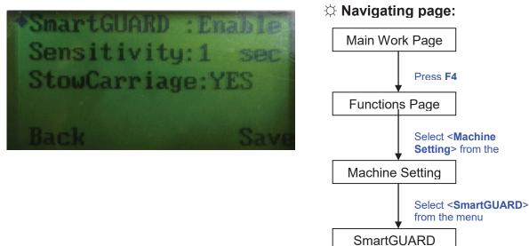
• **StowCarriage:** When set to "Yes", the lens carriage will move away from the source of the fire before automatic shutdown.
