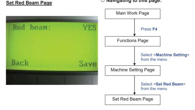
The Set Beam Page allows you to turn on or off the red dot laser pointer on the laser carriage. Enabling this function will indicate the exact location where the laser will fire upon.
