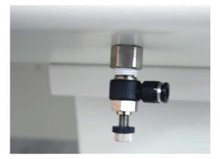
5) Take the unattached end of the ¼" air tubing (other end already connected to air compressor) and connect it to the air tube connector on the air assist valve. Make sure you press down on the air tube fastener when inserting the ¼" air tubing, to form a tight, secure attachment as indicated in the diagram below.
