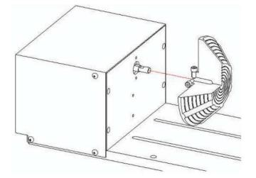
C. Assemble the smaller conical fixture onto the rotary attachment as shown below.
