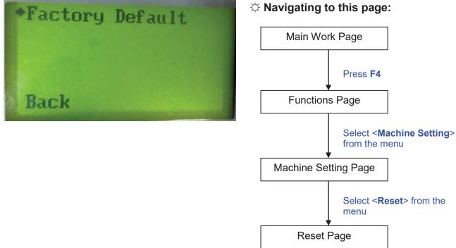
The Reset Page will restore machine settings back to factory default. Press ENTER to confirm the change, and restart the machine.
