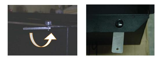
**CAUTION** Damage may occur to the system if you try to raise the work table without proper setting of the metal guard.
