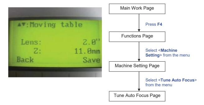
The Tune Auto Focus Page allows you to manually set the default auto focus distance / vertical height of the worktable (Z-axis) for when the Auto Focus button is pushed.
