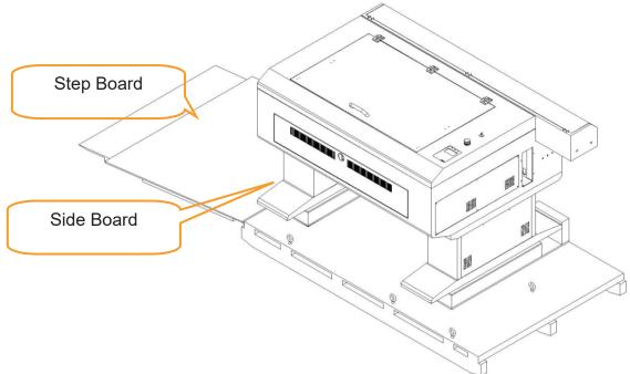
8) Carefully slide the machine off the shipping crate and position it into your work space.
