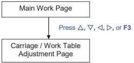
The Carriage / Work Table Adjustment Page allow you to manually increase and decrease the height of the work table (Z-axis). In addition, you can manually adjust the Y-axis and X-axis of the laser carriage.
