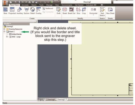
3. Set sheet size to match working area of engraver. Engraver working area can be found on the paper tab of the windows driver.
