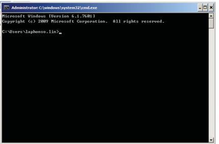
ii. Type "ping x.x.x.x –t" after the prompt symbol, (x.x.x.x is the IP address you set on the laser machine, ie: 192.168.100.101)., press "Enter" to run the "Ping" tool.
