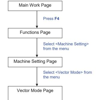
The Set Vector Mode Page allows you to adjust and balance vector mode's quality and speed settings based on your specific job. Speedy Vector Mode offers the highest output speed, sacrificing quality. Whereas Quality Vector Mode offers the highest quality, sacrificing output speed. Keep in mind that speed and quality are usually at a tradeoff. The system's default is Fine Vector mode, sacrificing some speed for higher quality.
