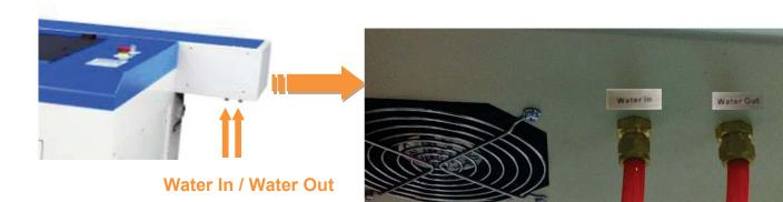
3. Connect the tubes to the water chiller.
