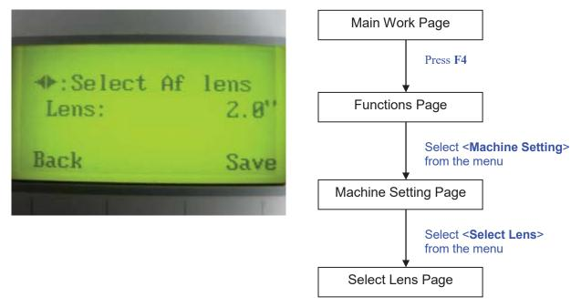
The Set Lens Page allows you to modify the lens setting after you have changed to a different focal lens. Remember to save your settings after you have made the proper changes. Now by pressing the Auto Focus button, the LaserPro MG380Hybrid will auto focus properly using the new lens setting. The LaserPro MG380Hybrid's default setting is <2.0>
