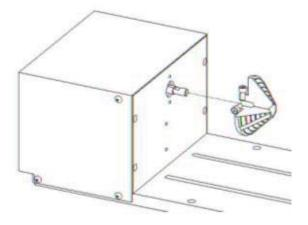
D. Use the flat surface as shown in picture below as a reference point and tighten the first screw against it. After doing so, tighten the second screw and the rotary attachment is ready for use.
