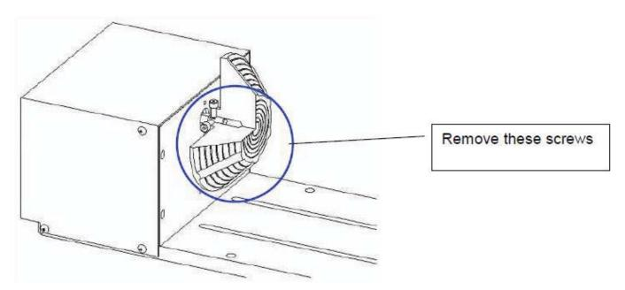
B. Detach the circular cylindrical cone by moving it in the direction of the arrow as shown below.
