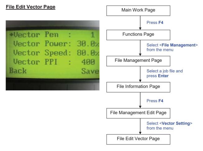
The File Edit Vector Page allows you to edit the vector pen, vector power, vector speed, and vector PPI, and power ramp settings for the selected job. These settings correspond to the same settings found on the LaserPro MG380Hybrid print driver. This page allows you to easily adjust these values to make immediate adjustments while processing your loaded jobs, even when you have disconnected your computer from the LaserPro MG380Hybrid.
