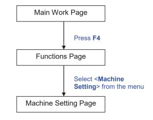
The Machine Setting Page allows you to access and modify a variety of your machine settings, including: Set Lens, Tune Auto Focus, Set Table Down, Set Red Beam, Carriage Lock, Set Command Mode, Save Position, Flash Memory, Set File Save Mode, Set Vector Mode, Tune Image Power, Set Laser Wattage, Set Fine Mode, Other, Reset.
