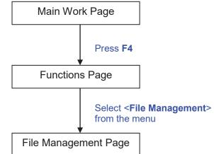
The File Management Page allows you to manage the files that you have loaded onto the LaserPro MG380Hybrid. You can scroll through your jobs, delete a selected job, delete all jobs, and go to the Link/DLink Page to set and arrange multiple loaded jobs into a single job queue for processing.
