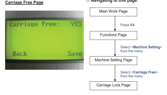
The Carriage Lock Page allows you to set whether the laser carriage is locked or free. If the Carriage Free setting is set to <YES>, then you will be able to manually move the laser carriage along the X and Y axis by hand with the top door open. Whereas setting the Carriage Free to <NO> will lock the laser carriage and movement or positioning can only be done by the control panel.
