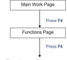
To recall the saved position, simply go to Functions page and press F4 again to recall the saved position. The lens carriage will be moved to the saved position and start subsequent jobs from this origin.
