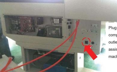
Plug the external **220V** air compressor to this power outlet to control the air assist function by laser machine driver and firmware
