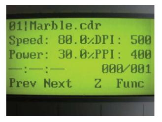
The main work page is the page that the LaserPro MG380Hybrid will default to upon startup and will be the "home base" for when navigating through the various functions of the control panel. This will be the page that is displayed when you are processing your jobs. This page contains specific job information such as the current job's name, Speed, Power, PPI, DPI, processing / remaining times, and jobs loaded.
