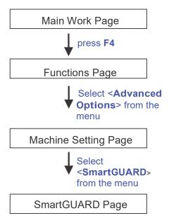
After optional SmartGUARD hardware installation, please enter the function menu on the control panel to enable the SmartGUARD fire alarm. Note SmartGUARD fire alarm system is not a fire extinguisher, but a fire detecting and alarm system.
