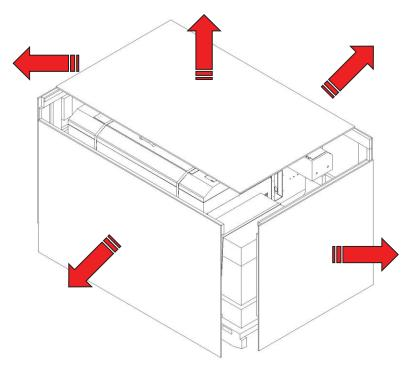
4) Use a slotted screwdriver or a suitable tool to pry the metallic piece as shown below. Once the metal piece has been pried straight as shown below, we can remove the metal strips and remove the wooden panels.
