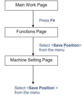
The Save Position Function allows you to save the current X-axis and Y-axis positions of the laser carriage and sets this position to be the origin for subsequent jobs.
