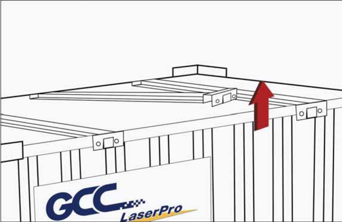
Step 5: Use a flathead screwdriver to pry loose the side brackets and remove them.
