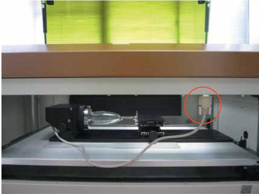
To load the object, you can use the enclose tools to widen or tighten the metallic claws. Simply insert the two metal pins into the holes on the turn-dial and turn it to widen or tighten the claws to hold the engraving object.
