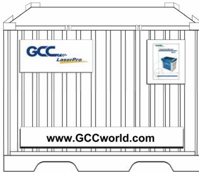
Step 1: Remove the 6 metal clips that secures the top panel to the crate by using a flathead screw driver
