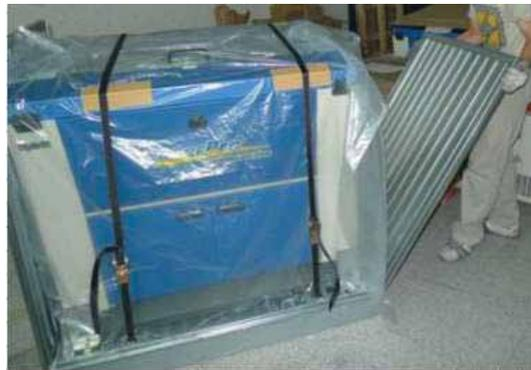
Step 4: Fix the four side boards by four corner brackets.
