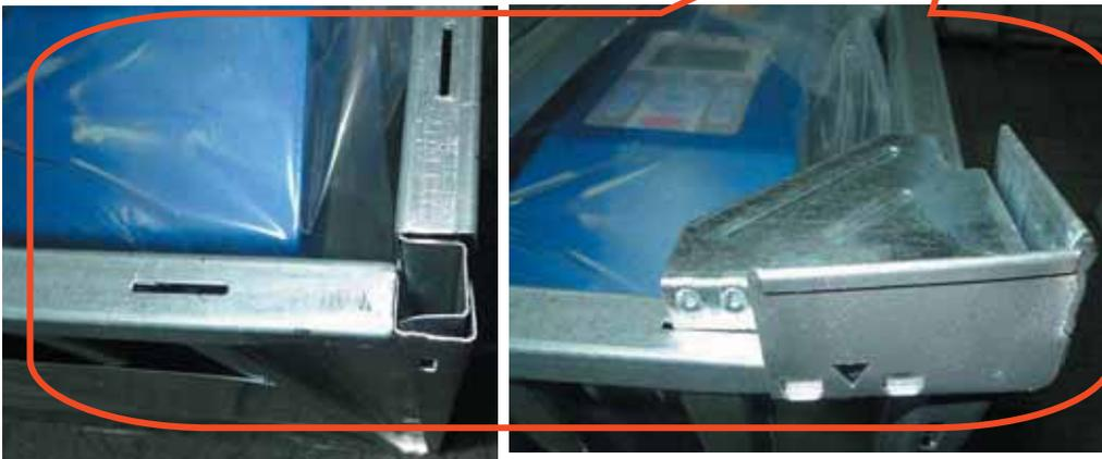
Step 5: Place the top cover on the top of the machine and fix it with the fixers.
