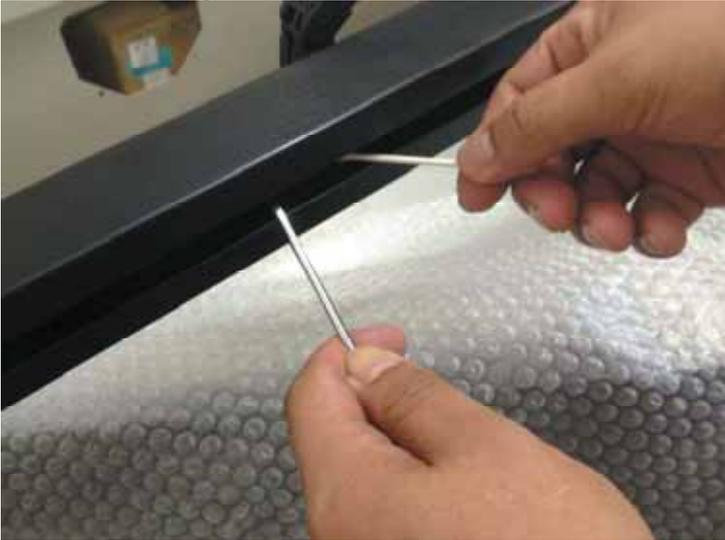
2. Use clean oil on cotton swab and then grease on linear guide (including top, bottom and surface of linear guide).
