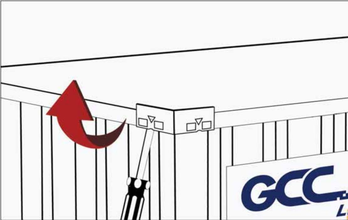
Step 6: Pull the front panel and lower it to an angle of about 45 degrees and then pull it away from the crate. Do the same for the rear panel.
