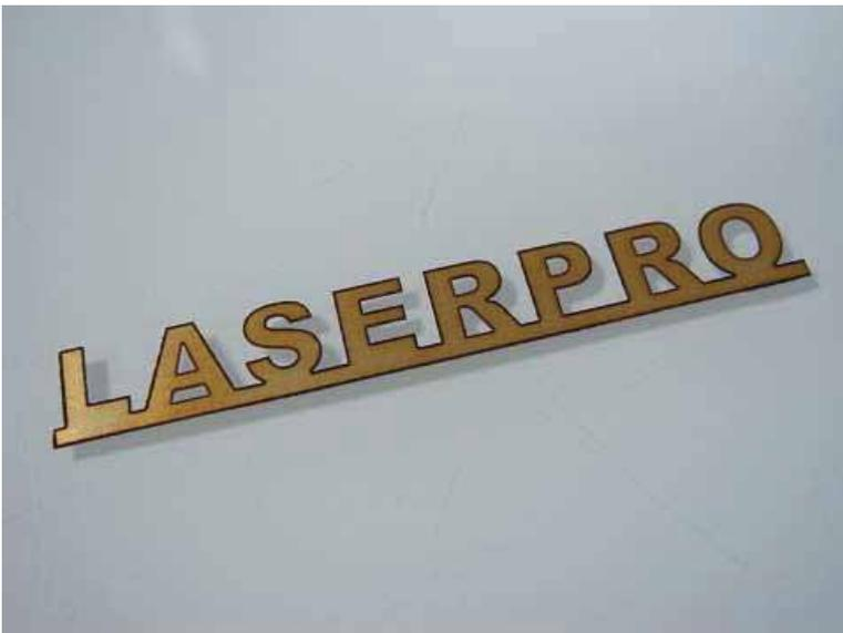
The LaserPro S290LS Print Driver determines which sections should be raster engraved or vector cut based on the outline width of that particular area or section of the design. In order to prep a particular section for vector cutting, you will need to set that object's fill color to white and set its outline thickness between 0.001" (0.025 mm) to 0.004" (0.1 mm) via the graphics software.
