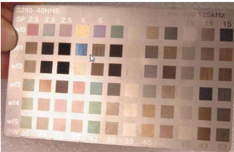
Firstly design a matrix with fixed speed/ power range, and frequency, change multiple waveforms as the key parameter, different colors can be marked by laser.
