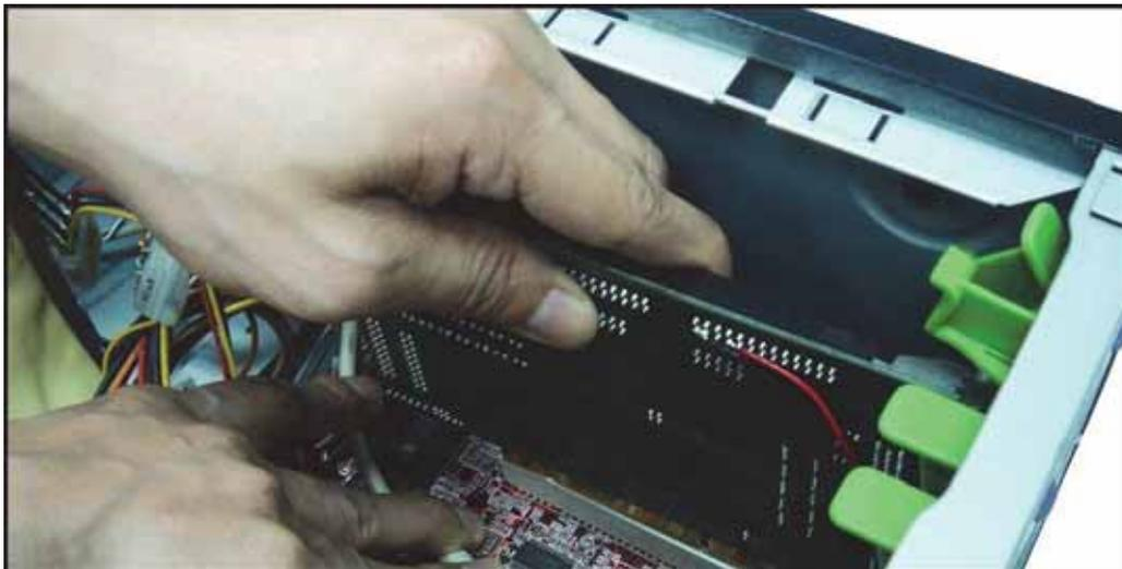
3) Connect the two 26 Pin Cables to the JF2 and JF4 slots of the PMC2 board
