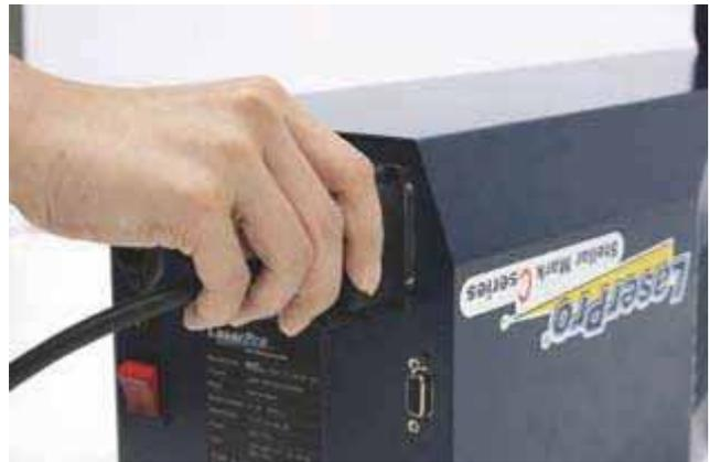
Step 3. Turn on the master power for laser Marker
