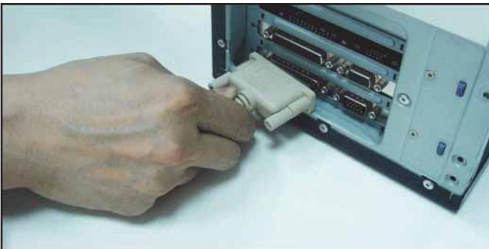
10) Connect the D-Sub 25 pin cable to the I/O interface
