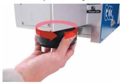
Use acetone if the lens cleaner will not remove the mark. Be careful not to scratch the lens. After the mark is removed, follow the steps used to clean residue marks in order to finish the cleaning.
