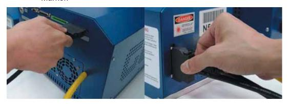
**Step 3.** Connect the USB cable between a PC or Laptop and the Control Unit.
