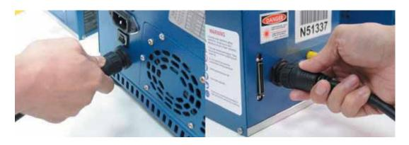
**Step 2.** Connect the SCSI cable between the Control Unit and Laser Marker.
